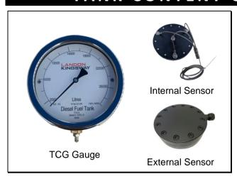
The Landon Kingsway TCG series calibrated hydrostatic tank contents gauge featuring capsule type movement for remote contents indication up to 30m. Individually calibrated to suit tank heights of between 600mm and 10m height or diameter depending on the density of the liquid to be measured.
